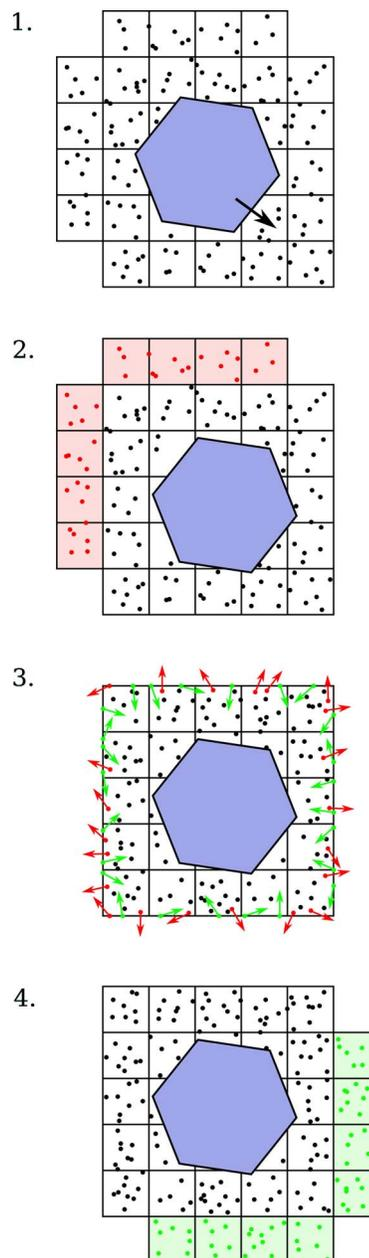
FIG. 1. Illustration of the ideal gas algorithm. (1) Propagate crystal atoms (blue). (2) If necessary, remove cells and gas particles therein that are no longer needed (red). (3) Propagate gas atoms and remove those (red) that leave the atmosphere. Put new gas particles (green) on the surface and propagate them into the atmosphere; remove those (red) that end up outside. (4) If necessary, add new cells and fill them with gas particles (green).
