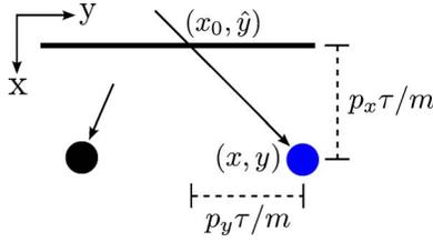
FIG. 3. Illustration of the variable transformation (30),  $z$ -direction not shown. The arrows indicate particle velocities, with arrows starting at particle positions one time step in the past. The blue gas atom was injected from the point  $(x_0, \hat{y})$  on the surface, and propagated for a time  $\tau$  to its final position  $(x, y)$ . The other particle could not have reached its position through an injection event.
